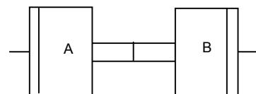
$$P_1 V_1^\gamma = P_2 V_2^\gamma \Rightarrow P_0 V_0^\gamma = p_1 (2V_0)^\gamma \Rightarrow P_1 = P_0 \left( \frac{V_0}{2V_0} \right)^\gamma = \frac{P_0}{2^\gamma}$$
