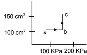
(b) Work done = Area enclosed under the graph  $50 \text{ cc} \times 200 \text{ kpa} = 50 \times 10^{-6} \times 200 \times 10^3 \text{ J} = 10 \text{ J}$
