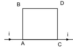
20. For AB  $B$  is along  $\odot$   $B = \frac{\mu_0 i}{4\pi r} (\sin 60^\circ + \sin 60^\circ)$
